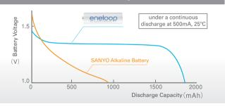
eneloop can be used for a long time at a constant voltage
