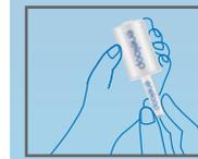
Just plug the eneloop into the adapter and you can use it in your equipment. Of course the adapters only adapt the mechanical dimensions of the eneloop.
